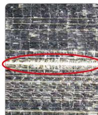
Due to the new design of chip-splitting there is no visible mark as happens when using a conventional milling tool. The result is an excellent surface quality.
