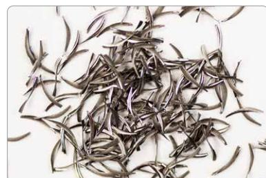
Due to the chip-splitting the chips are short and easily evacuated. The result is long tool life.
