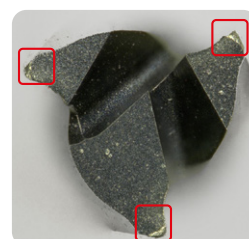
Edge wear after 276" (7 m) in CoCr alloy
