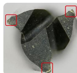
Edge wear after 276" (7 m) in CoCr alloy
