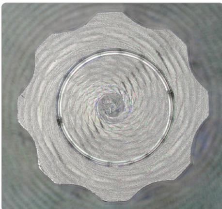
The material-specific geometries cut the material so perfectly that burr formation is nearly avoided.
