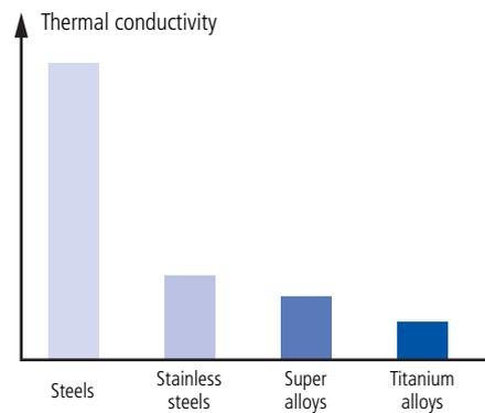
Titanium and heat-resistant alloys are notable for their high toughness and low thermal conductivity. Machining produces extreme temperatures on the cutting edges, resulting in high tool wear.
