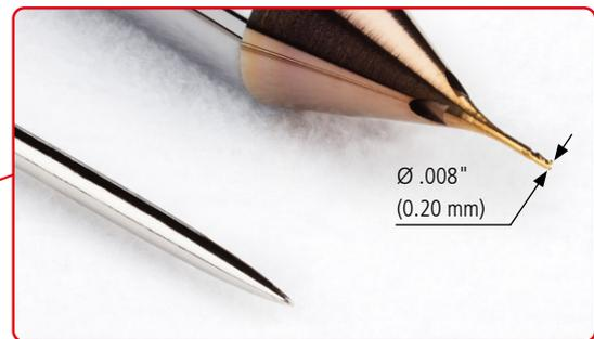
Miniaturisation presents the challenge of realising complex geometries with diameters less than .039" (1 mm). The smaller the tool's cross-section, the more challenging it becomes to mill complex geometries while ensuring that quality requirements and tolerances are met.
