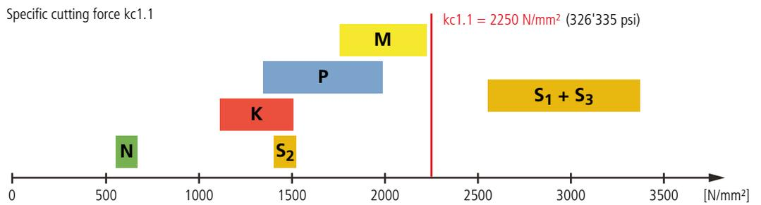
Close attention must be paid to the different mechanical properties of various material categories\* in micro-machining. The cutting forces of superalloys and CoCr alloys are up to 45% higher than those of stainless steel and titanium ( $kc_{1.1}$  values). As a result, the cutting edge is subjected to high mechanical stress, leading to chipping.
