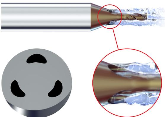
The innovative, patented cooling concept solves this problem. The cooling lubricant is applied directly and extensively to the cutting edges, thereby allowing the heat to dissipate. The result is higher cutting speeds and a significantly higher material removal rate.
