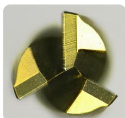
Edge wear after 787" (20 m) in CoCr alloy
