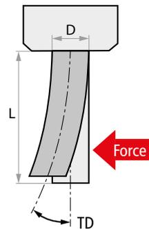
Tool deflection constitutes a significant problem for small diameter milling operations, which is further exacerbated when processing difficult-to-machine materials due to the higher cutting forces involved.
