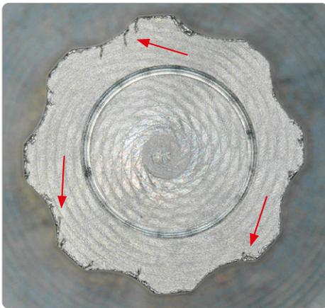
Another challenge is the massive burr formation, which is more pronounced when milling challenging materials.
