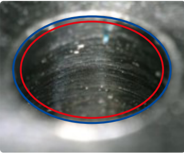
Requested diameter (i.e: Ø.0787" (2 mm)) Machined diameter (i.e: Ø.0803" (2.04 mm))
